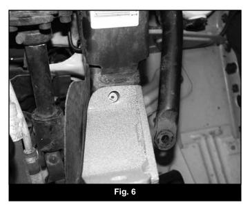
14. With the hole position marked for the track bar bracket, rotate the bracket out of the way and drill a 7/16" hole at the mark. Only drill through the bottom surface of the frame. Attach the track bar bracket to the bottom of the frame (Fig 7) through the new hole with a 7/16" x 1-1/4" bolt, 7/16" SAE washer (BP 753) and provided nut tab (01356). Use Loctite on the bolt threads. Leave hardware loose.
