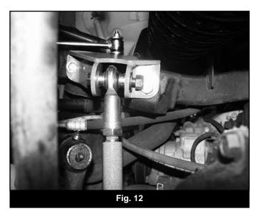
27. Be sure to cycle the suspension from full compression to full droop while cycling the steering from lock to lock. This should identify any clearance issues. Recheck all fasteners after 500 miles.
