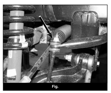
2. Install the sway bar link extension onto the factory sway bar link. Attach the assembly to the sway bar with the factory bushing, cup washers, and 10mm bolts (Bolt pack #654) and Loctite on threads. Tighten bolt until bushings begin to deform. It is NOT necessary to over tighten the bolt.
