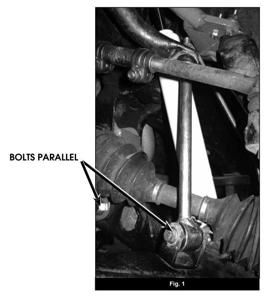
3. With the links completely installed, tighten the 3/8 hardware to 30 ft-lbs and the 5/8" hardware to 75 ft-lbs.
