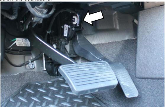
3. Connect supplied wiring harness to the sensor and connect the other end to the factory wiring harness. Secure harness with zip ties so that it does not interfere with pedal operation. Removal of the knee bolster may ease installation.
