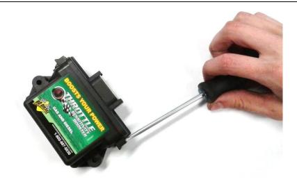
5. Connect circuit board to the wiring harness and keep away from metal objects that might cause a short circuit. Ensure the sensitivity "SETTING" switch is set to the default position of "STOCK".
