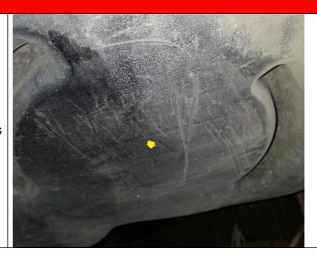
2. Now, create a 3" hole by drilling through the tank using the hole saw. If fuel remains in the tank, place a drain bucket below with a large enough capacity.
