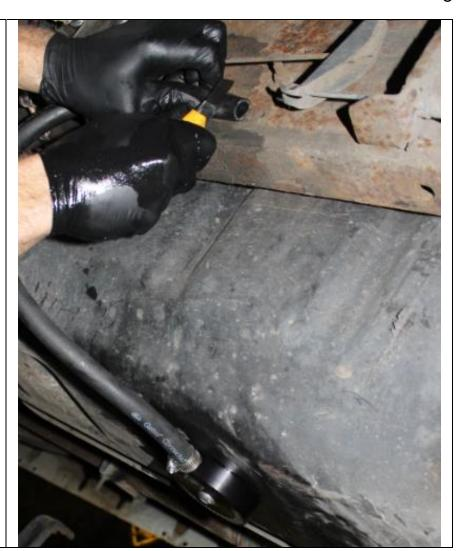
13. If desired, remove the old fuel supply line from the pickup and cap using the hose plug/clamp/fuel hose as shown. The larger of the two lines will be the supply, either 3/8" or 1/2"
