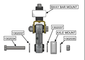
7. Center U-bracket rod in the sway bar and torque Nylock nut 10-12 ft/lbs (16mm).
