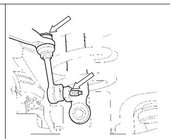
Lubricate (2) Polyurethane bushings with the supplied lubrication and press into cast link (1312050) using an arbor press. Then insert steel bushings into the assembly.
