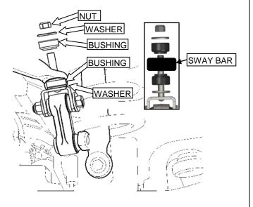
6. Assemble the end link assembly using the two supplied washers and bolt. Then slide the assembly into the axle mount and secure into position using the supplied washer and Nylock nut and tighten finger tight.
