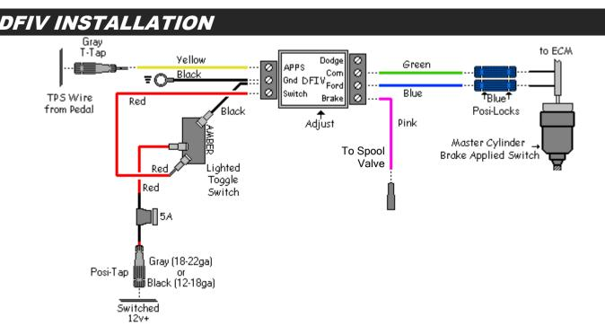
**CAUTION:** Before installing any wiring modifications or equipment ensure to disconnect the battery Ground (Negative) terminals on all the vehicle batteries as damage to the vehicle's ECU and/or installed components may result.
