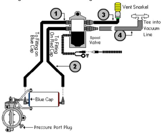
Find the hose running from the vacuum pump to the power brake booster. Cut this hose just before the vacuum manifold and install the 3/8" plastic tee (w/hose attached) to the two pieces of hose. Attach the free end of the supplied hose to the unused barb fitting on the Spool Valve (#4).
