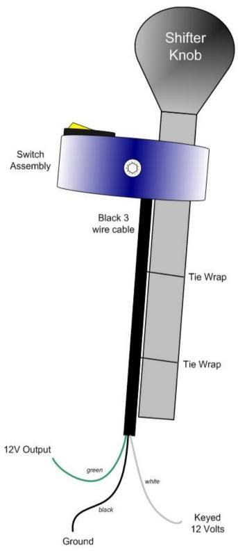
a 14/16ga) and connect an appropriate Posi-Tap connector to it (green for 10/12ga and black for 14/16ga wire). Connect the white wire of the rocker switch assembly to this Posi-Tap.
