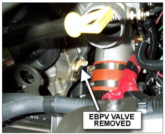
NOTE: ON CALIFORNIA MODEL VEHICLES THE EBP VALVE WIRING MUST BE CONNECTED TO ENSURE THE ECM DOES NOT SET AN ENGINE TROUBLE CODE.
