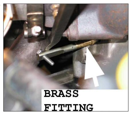
to loosen it, then taken out with the use of a swivel socket.
