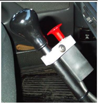
Connect the white (or green) wire to the "NO" (Normally Open) terminal of the micro switch (12 valve) or to the "Switch" terminal on the DFIV Module (24Valve).
