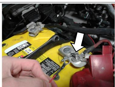
30. Carefully secure the wiring around the engine bay with zip ties to ensure it does not come in contact with hot surfaces.
