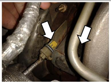
25. Connect the BD VVB wiring harness to the turbo solenoid and to the OE wiring.
