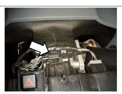
8. Use wire ties to secure the wire down the bottom of the steering column beside the OE harness.
