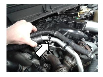
22. Undo the transmission and engine oil dipstick tube bracket from the intake manifold by removing the 8mm fastener.
