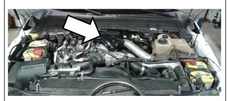
20. Disconnect the wire connection from the MAP sensor on the top of the intake manifold.
