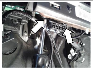
10. Install the OBD connector from the BD VVB kit in place of the original and reinstall the screws.
