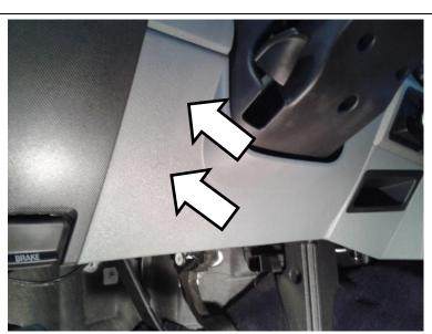
Route the black wire with ring terminal to the driver side battery negative terminal.
