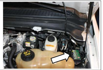
9. Connect the in-cab wiring harness to the control module in the engine bay by plugging in the small eight pin white connector.
