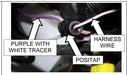
6. Install push button switch and connect to the BD wiring harness.
