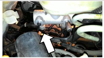
Disconnect the turbo vane actuator. Connect the BD harness to actuator and OE plug.
