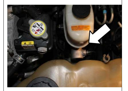
**Note** There are two connectors on the bottom of the master cylinder. The correct connection is the one towards the front of the vehicle.
