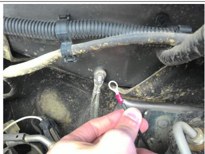
5. Route the VVB switch wire through the firewall from the engine bay into the vehicle cab.
