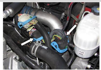
4. Connect the ground wire from the module to the body ground on the firewall, or to another body ground.
