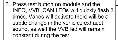
NOTE: The LED's at the two relays will also light up when the turbo vanes are engaged.
