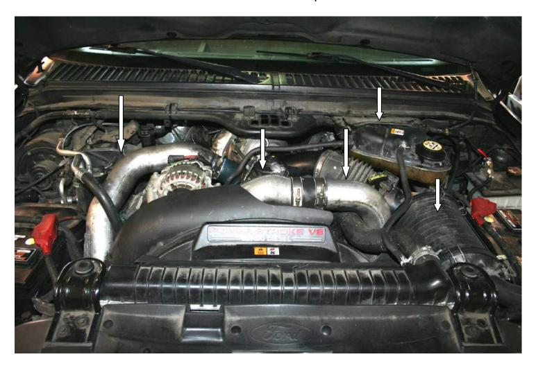
Remove the air cleaner assembly by disconnecting the MAF sensor and Filter Minder device. Then remove the ribbed hose, then the air box. Remove the two (2) 8mm bolts securing the hard tube. Then remove the breather tube from the vent on the driver side rocker cover. (NOTE: Wiggling and pulling out on the tube will help in removal).
