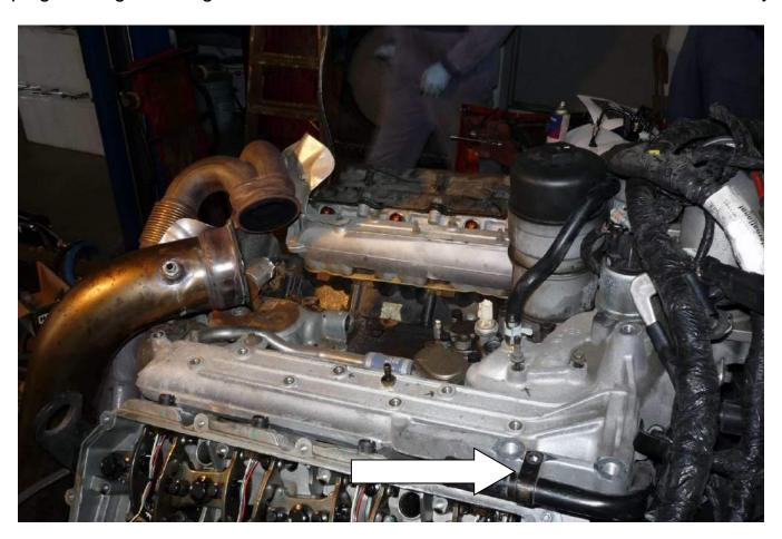
NOTE: Bend back the tab on the rigid metal tube at the RH side of intake manifold to allow manifold to clear.
