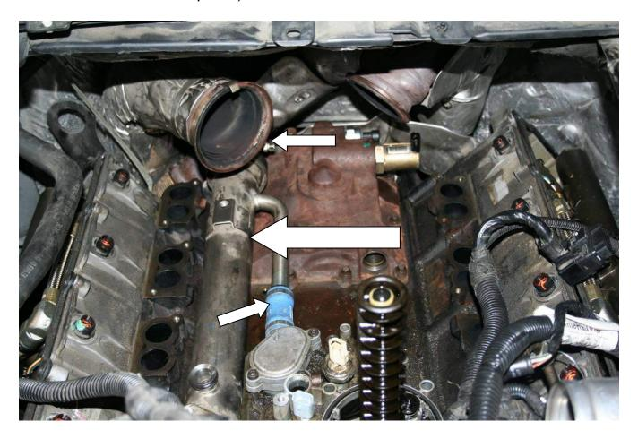
Remove the EGR cooler by disconnecting the clamp at the exhaust feed pipe then remove the coolant hose by first twisting about 90° and sliding back along the cooler tube.
