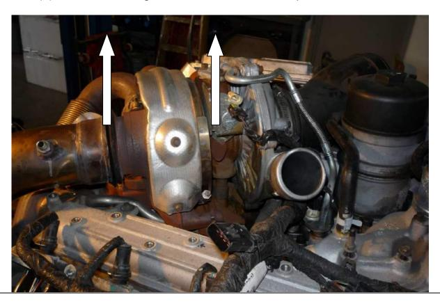
11. Reconnect fuel filter wiring connectors and fuel lines then fuel filter housing.
