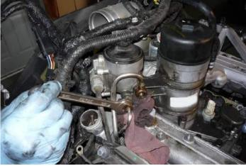
12. Reinstall the oil filter and EGR valve, service both as required.
