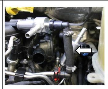
57. Locate OEM fuel return quickdisconnect (seen here with blue latch), and remove. This is done by lifting the locking
