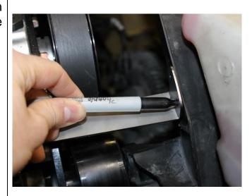
47. Drill two(2) 6mm(.236in) diameter holes on marks made in previous step.
