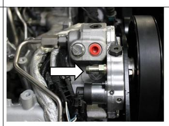
39. Install 1500728 Banjo fitting, 1502015 Banjo bolt, and 1502019 seal washers. Assemble hand tight as shown.
