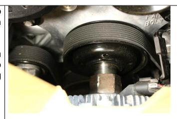
44. Torque fan bracket bolt to 18 ft-lbs, using a 13mm socket and reconnect fan clutch connector.
