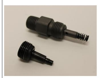
21. Install new output fitting with spring and ball bearing. Torque to 56 ft-lbs, using a 17mm socket.
