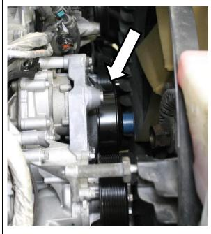
Using 13mm socket, remove three
