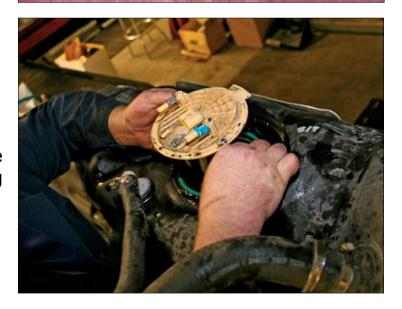
Raise fuel tank back up into vehicle and reconnect all connections. Secure the tank to the vehicle.
