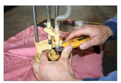
Use the supplied 3/8" hose and stainless hose clamp to attach the hose to the 3/8" barb.
