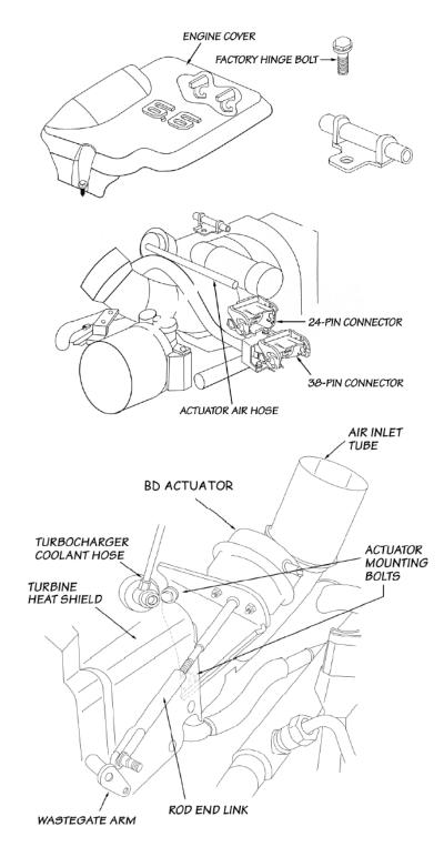
Using the two 12mm bolts, mount the BD actuator in place of the factory wastegate. Securely tighten the two bolts.
