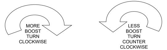
To increase the boost pressure, you will have sufficient energy to drive the turbo faster. Once you have turned the rod to the desired position, re-install the circlip and lock the jam nut.
