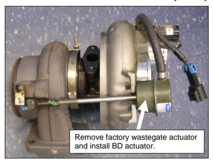
locknut. Apply air pressure to the wastegate diaphragm; this should stroke the rod end forward. Align the wastegate arm hole with the BD rod end and insert and lock into place with the supplied cir clip. Once the clip is in place you can then tighten the mounting nuts.
