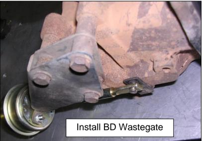
the rod end forward. Align the wastegate arm hole with the BD rod end and insert and lock into place with the supplied cir clip. Once the clip is in place you can then tighten the mounting nuts.
