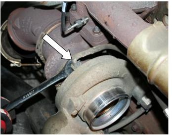
On 2005-2007 trucks, unplug the wastegate solenoid connector
