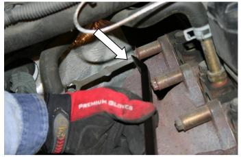
Remove the manifold heat shield with a 15mm socket
