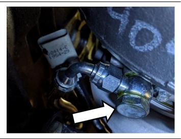
Form the supplied oil drain into shape and install onto the turbo oil drain with provided gasket. Transfer the oil drain bolt from the stock turbo.
