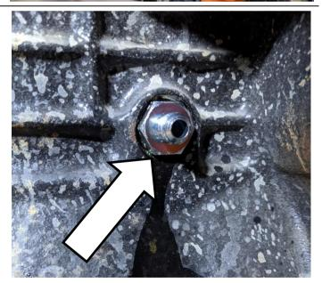
Loosely install the Banjo to JIC fittings in the bottom of the turbocharger.
