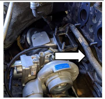
Install the manifold and gaskets onto the engine and turbo. Torque manifold bolts and nuts to 33ft-lbs.
