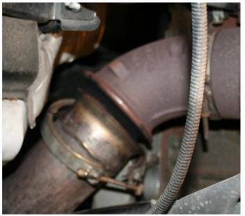
Remove the turbo oil drain with a 10mm socket and pull the line out of the engine block
