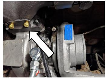
Secure the coolant like to the manifold using the provided bracket.
