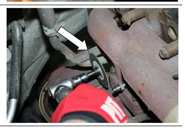
Remove the turbo oil feed from the turbo
