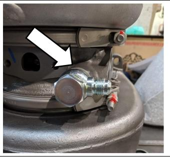
Loosely install the coolant line (1407023) as shown.
