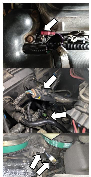
Connect the main harness to the fuel bowl heater by plugging it inline. This provides power to the kit
