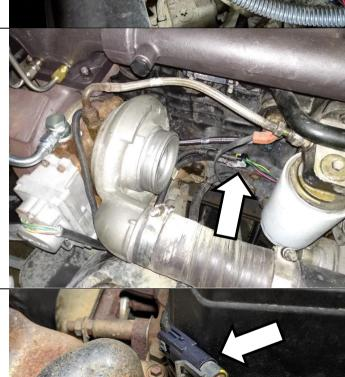
2004-2007 Models Connect the main harness to the coolant temperature sensor by plugging it inline.
