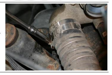
Pry off the metal lock from the rear manifold bolts. Remove the heater pipe bracket.
