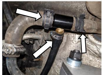
Install the JIC to Barb fitting. Secure the hose onto the fitting.
