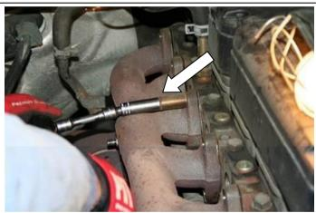
Remove the turbo/manifold as an assembly.
