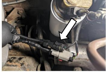
Install the oil feed line. Tighten at both ends.
