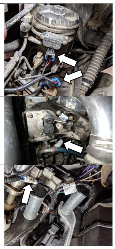
Route the RED and PINK wires from the toggle switch kit (1407038) from inside the cab to under the hood near the VGT control module.
