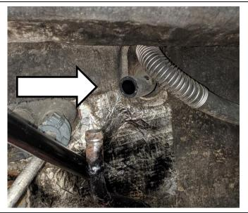
Install the supplied the tee fittings (1900075, 1407033) as shown. Secure both sides with supplied spring clamps.
