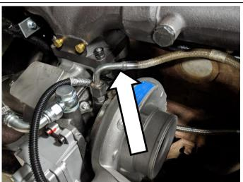
Install the boot at the turbo outlet and re-install your intake system and airbox.
