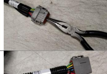
Remove the two seal pins in pins 10 and 11 by pulling them out the back with a pick or small screwdriver.
