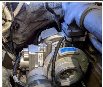
Secure the coolant line to the JIC fitting in the engine block installed earlier.
