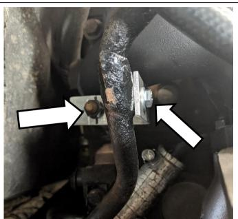
Install the provided exhaust outlet elbow to the turbo and the exhaust downpipe. Reuse your stock downpipe clamp. Turbo to exhaust elbow clamp is provided in the kit.
