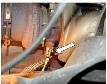
Cut the heater pipe bracket close to the manifold (leave enough of the bracket attached to the pipe to re-affix later)
