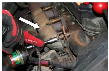
Remove the remaining manifold bolts using a 13mm socket
