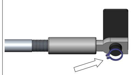
4. You can now un-thread the rod end from the shaft. Note that you will need to release the jam nut if there is one.
