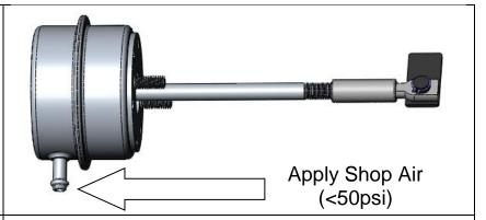
3. Once the tension is released you can remove the retaining ring, and push the rod out of the center hole.
