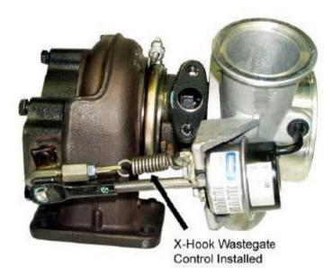
Once the adapter plate is attached, proceed hook the spring assembly to the adapter plate while also hooking the "J" hook around the waste gate control arm. Before doing this ensure the tension nut is loose and evenly spaced from either end of the hook and the "eye" bolt. Also ensure that the lock nut is also furthest away from the tension nut as possible.
