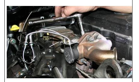
10. Remove the EGR flow direction valve from the vehicle.
