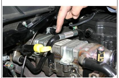
14. Remove the coolers two rear bolts that attach it to the exhaust system (15mm)
