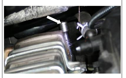
15. Prop the cooler above the studs and push towards the cab holding the other coolant hose to release the oring fitting to remove the cooler from the vehicle.
