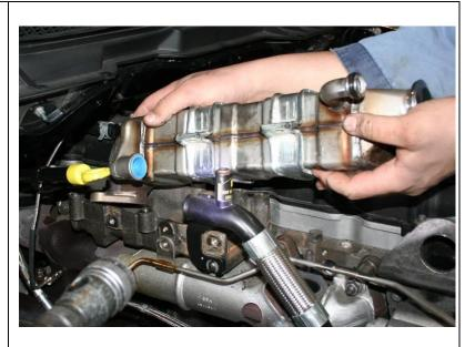
16. Remove the cooler mount bolts to the head (13mm socket) and remove the cooler mount from the vehicle.
