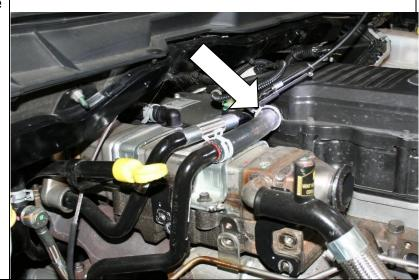
12. Remove the four bolts for the cooler and the nut that holds the transmission dip stick tube in place. Then nudge the tube out of the way to access the nut under the dip stick bracket.
