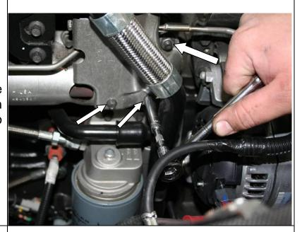
7. Remove the three bolts for the stepper motor bracket (10 mm) socket and prop the bracket on the cooler.
