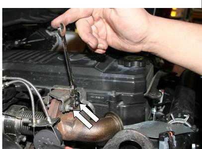
5. Remove the air box and intake hose. Remove the air filter inlet hose from the turbo inlet.
