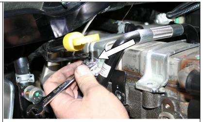
13. Remove the EGR coolant hose from the cylinder head to the cooler. (All bolts should be already removed) the hose is held in by orings. Remaining coolant will drip out.
