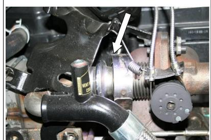
9. Using a (15mm) socket remove the outer nut for the exhaust flange of the flow valve at the manifold.
