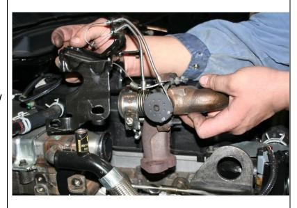
11. Remove the bolt that holds the CCV hose to the cooler then disconnect the clamp at the valve cover to remove the hose assembly.
