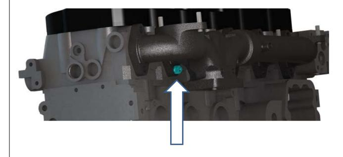
3. The five exhaust manifold cap screws with studs are used at the No. 1 and No. 2 cylinder locations for the heat shield mounting and one on the rear lower corner of the manifold for the cabin heater tube bracket.
