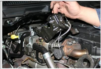
8. Loosen the clamp (11mm) that connects the EGR Flow Direction Valve to the cooler and slide the clamp towards the valve.
