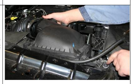
6. Remove the top bolt from the lower heat shield (10mm) then the other two (8mm) bolts to release the lower heat shield.
