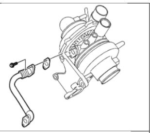
3. Install the oil feed pipe, washer, and bolt.
