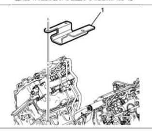
5. Install the turbocharger with the oil return pipe.
