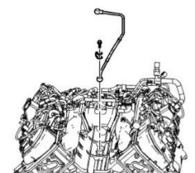
4. Install the turbocharger lower heat shield.
