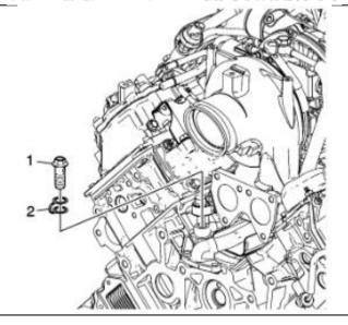
12. Install the turbocharger heat shield and bolts. Torque to 9 Nm (7 lb ft)
