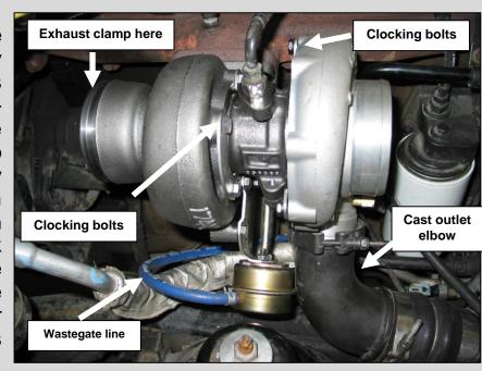
A new compressor outlet oring has been provided. Lubricate the oring and install between turbo and outlet elbow. Re-use the factory V-Band Clamp. Adjustment of the first intercooler boot may be required for a proper fit.
