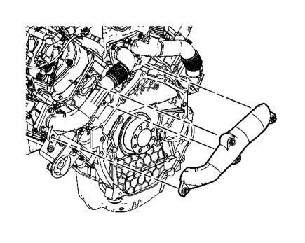
12. Using 12mm 12point socket wrench remove the driver side up pipe bolts.
