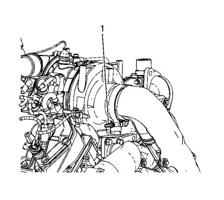
3. Remove turbocharger exhaust pipe to bracket bolt (#1). Remove the turbocharger exhaust pipe. If this is the OEM pipe you will discard as you will need an aftermarket one.
