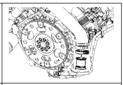
24. Re-install the turbocharger heat shield and glow plug controller if removed.
