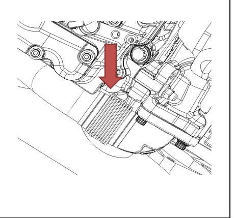
9. Tighten the exhaust up-pipe bolts in the sequence shown. Torque the bolts to 53 Nm (39 lbft)
