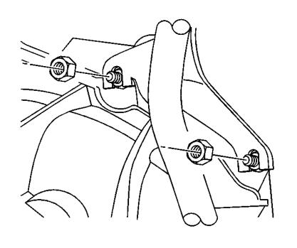
If using an OE/Stock turbocharger exhaust down pipe, remove the heat shield bolts and heat shield.
