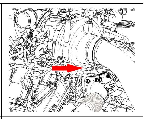
22. Re-install the transmission fluid fill tube. Install fluid fill tube to bellhousing nuts. Torque the nuts to 18 Nm (13 lbft).
