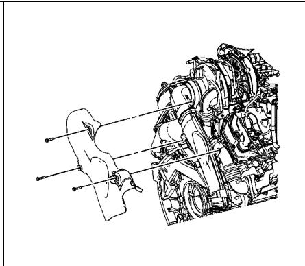
Using 12mm 12 point socket wrench remove the passenger side up pipe bolts.
