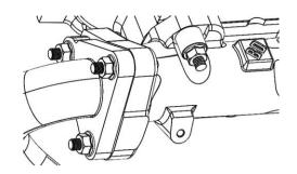
Install the manifold to EGR gasket (HC3Z-9E464-A) to the EGR tube.
