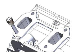
Install and torque new M8x1.25x35 studs (FT-11559036) into the end of the manifold.
