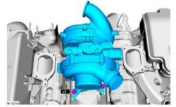
Install the cross over pipe gasket (BC3Z-6N640-A) and cross over pipe using the supplied flange lock nuts (FT-11508940).
