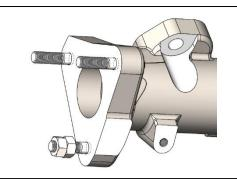
Install the manifold gasket (FC3Z-9448-A) and longer BD spacers (1403009) and locking flange nuts (FT-11508940). Torque the manifold using the following sequence:
