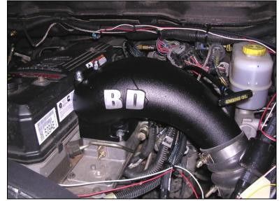
Move the intake around so that it is not touching anything and secure the intake with the supplied nuts. that the 12mm JIS nuts should be mounted to the smaller studs on the driver's side of the intake, while the 13mm Acorn nuts should be mounted to the longer studs. Be sure to place the washers underneath the Acorn nuts.
