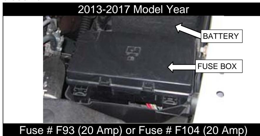
11. With the fuse box closed, mount the control module on top of it using the supplied Velcro.
