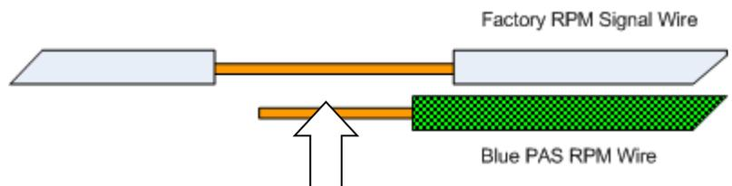
Solder the connection and then wrap and seal with electrical tape
