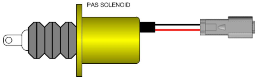
8. Next on the wiring harness, connect the BLACK and RED wires to the respective battery connections.
