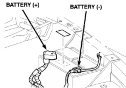
10. For the last connection you will need to locate ignition power. This will power the automatic over speed control box LED switch. Note the unit can still be activated manually with the switch at any time. Locate the fuse panel in front of the driver's side battery. Remove the cover. Locate appropriate fused ignition power circuit. Connect yellow wire with flag connector to this new connection. Route wire out of fuse box and close lid.
