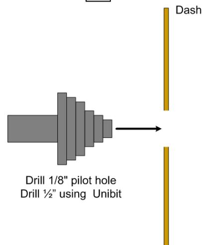
5. Once you have the mounting hole drilled, crimp the switch connectors to the switch wires and install the correct switch wires to the correct switch terminals, then insert the switch into the dash from the backside.
