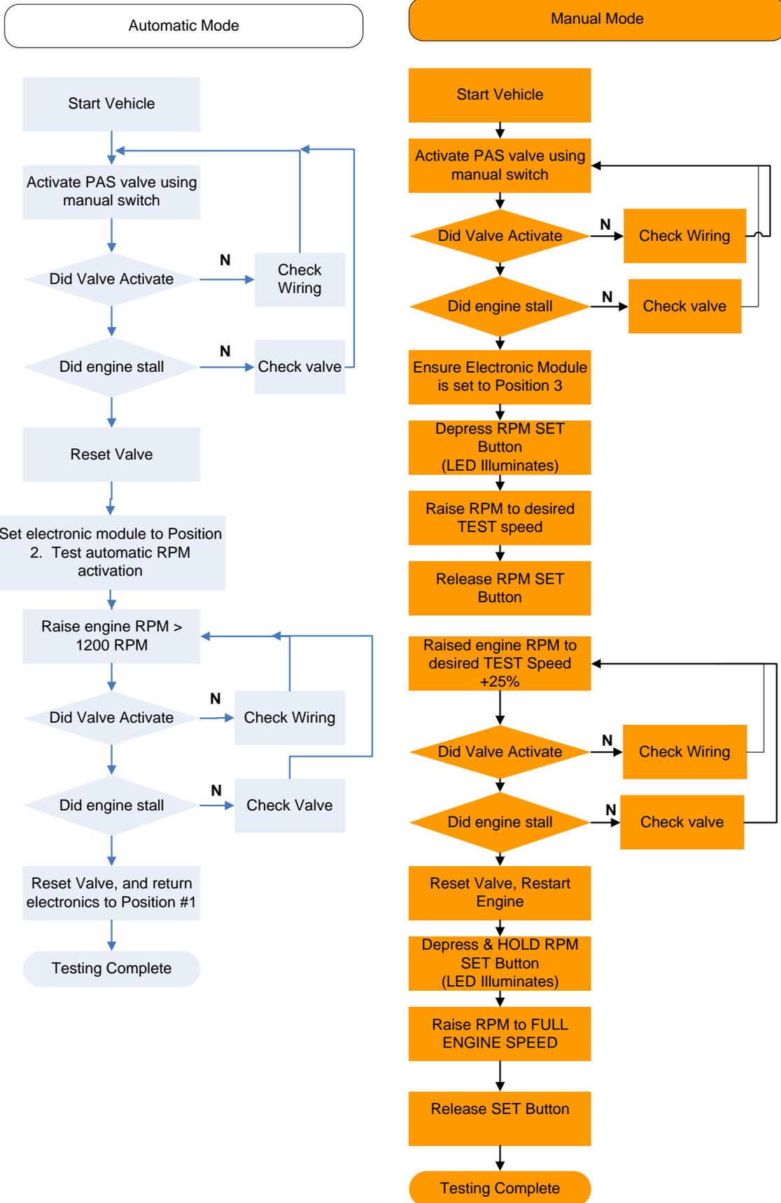
**TESTING FLOW CHART without OVER SPEED ELECTRONICS**
