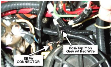
**NOTE:** After installation, ensure to replace the intercooler hose and clamps. Reattach the MAP sensor hose and wiring connector. Check all connections for security and tightness and secure all wiring to ensure they are out of the way of moving and heated items.
