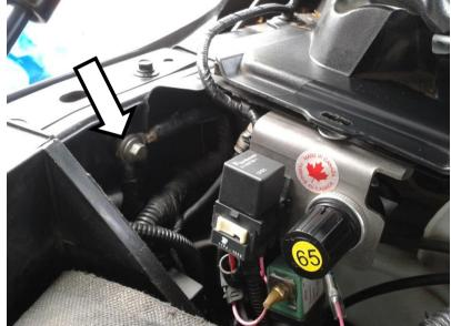
Connect the main power feed to the passenger side positive battery terminal clamp.
