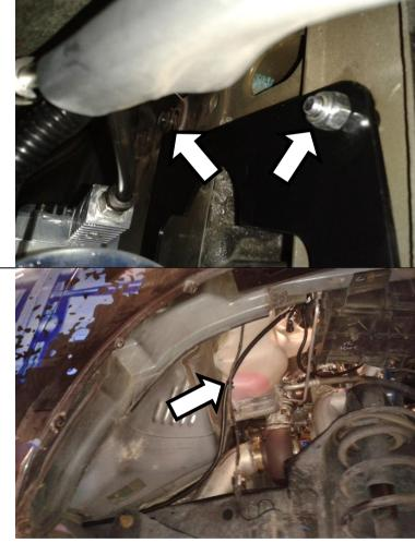
While the fender liner is off, double check that the air tubing assembly installed in the earlier section is well clear of the exhaust pipe, turbocharger and moving suspension components.
