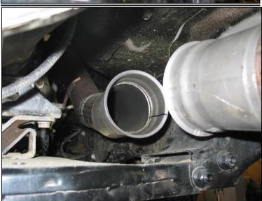
Ensure the exhaust brake and rear exhaust sections are pushed all the way forward on the front pipe so that the front adapter flange is up against the stop that is on top of the front pipe section then WELD the front adapter in place. Install the rear adapter to the pipe using the supplied band clamp.
