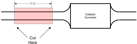
Clean off the cut ends of the intermediate pipe with a file to remove burrs left from cutting and then insert the adapter pipes onto each end of the now exposed pipes.
