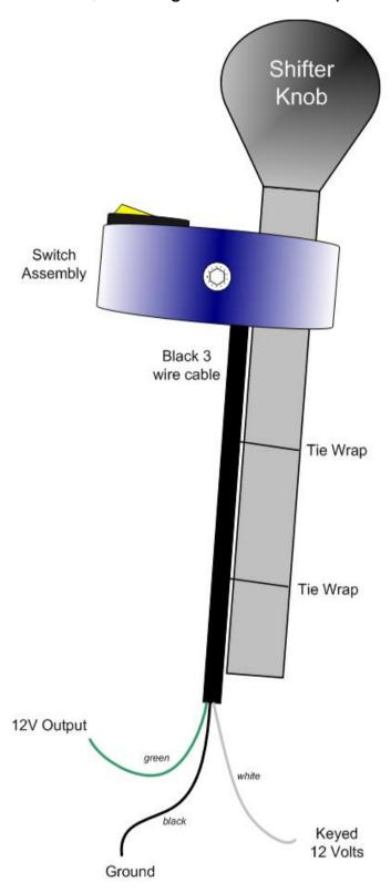
Locate one of the ignition switched power fuses in the fuse panel underneath the steering column. Traditionally this wire will be pink with a white tracer. Use a voltmeter to check the voltage of the wire. Use the supplied fuse tap to supply ignition switched power to the "Keyed 12 Volts" (white) wire of the rocker switch assembly.
