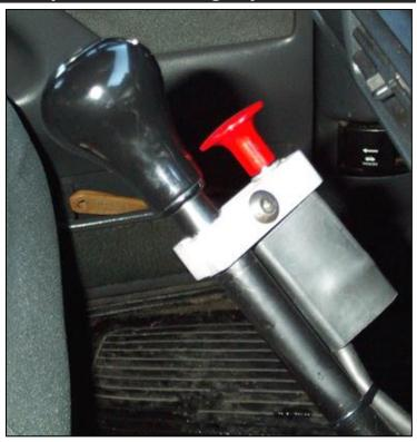
Connect the white (or green) wire to the Tan brake activation wire leading to the ECM. Connect the black wire to a nearby ground source. See page 17 for wiring diagram.
