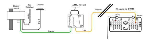
This switch relay is **not required** when wiring the exhaust brake with the push-pull style switch.
