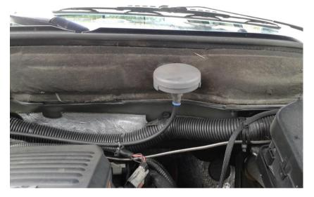
Locate the 1/8" tube from in the air tubing assembly that leads to the brake valve. This will be installed in the output from the air regulator assembly on the bottom of the solenoid.
