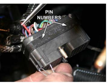
The two wire leads from the regulator assembly harness (with the ECM pins precrimped) can now be plugged into the ECM. Insert the tan wire into Pin #39, and the black wire to Pin #42. They should snap into place. Once this is complete, you can re-install the ECM plug. Secure the wiring loom using the supplied tie wraps.
