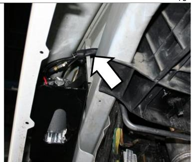
Secure the compressor in place by reinstalling the hood hinge bolt through the compressor bracket. Then install the nut and bolt to hold the front of the bracket.
