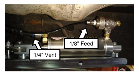
Route the air tubing assembly along the frame rail and secure with wire ties to the existing wiring harness.
