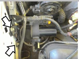
Remove the small electric vacuum pump from the stock bracket by removing the small screws. Reinstall on to the supplied relocation bracket. Trim the rubber ends on the three vibration dampers to clear when reinstalling. Install on the passenger side of the radiator support bracket with the two bolts and washers provided.
