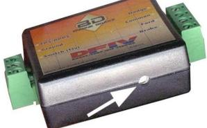
With the throttle at idle, start the engine and turn on brake switch. Then, using a small flat bladed screwdriver, turn the small adjusting screw in the DFIV Module counterclockwise or clockwise until the test light JUST turns on.
