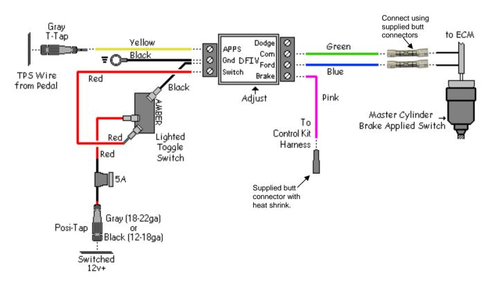
Remove lower section of dash, under the steering column, and mount the DFIV module to the cross member under the steering column. Connect the Black wire from the DFIV module to a good ground.
