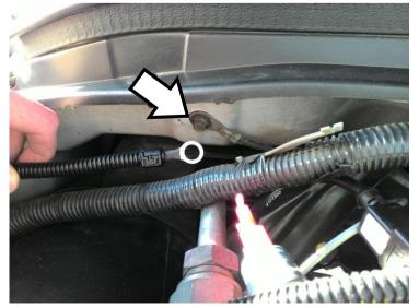
Connect the ring terminal on the red wire to the passenger side positive battery terminal (The negative battery leads should not yet be connected at this time).
