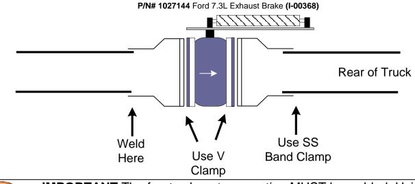
**IMPORTANT** The front exhaust connection MUST be welded. Using a band clamp or conventional exhaust clamp on this joint will cause leaks and will not retain full exhaust brake pressures.
