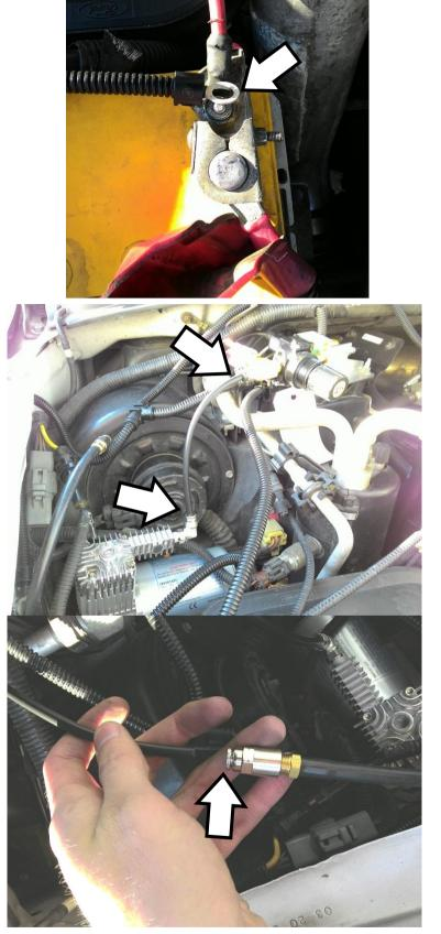
Locate the air tubing assembly previously installed on the brake valve air cylinder. Trim if necessary and install the 1/8" tube onto the outlet of the air solenoid. The other 1/4" line in this assembly is a vent for the air cylinder and may be installed in the same location as the air compressor inlet air filter.
