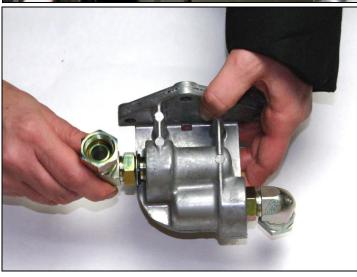
Install the two **90° ORB fittings** (1604046) into the filter head (<u>do not</u> use pipe sealant). When installed, the fittings need to point toward the front of the vehicle. For ease of installation, we recommend assembling the fittings on the filter head on a work bench before installing it onto the vehicle.
