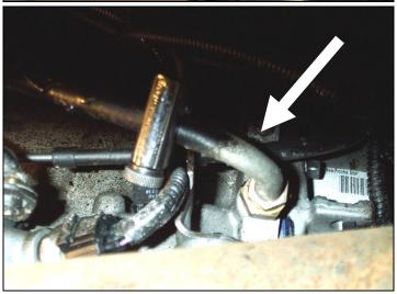
Locate the oil cooler line towards the rear of the transmission.
