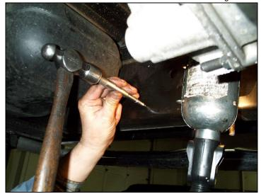
To allow for easier drilling, center-punch the two marked spots for the mounting bolts.
