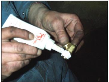
Install the two  $\frac{1}{2}$ " hose x  $\frac{1}{2}$ " NPT barbed fittings (1604047) into the 90° ORB fittings (1604046) using some pipe sealing compound or tape to the threads of the brass barb fittings only.
