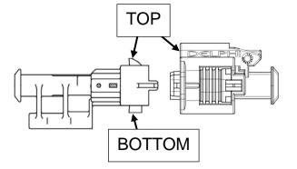
Connect the module to the gray plug from the transmission/engine wiring harness.
