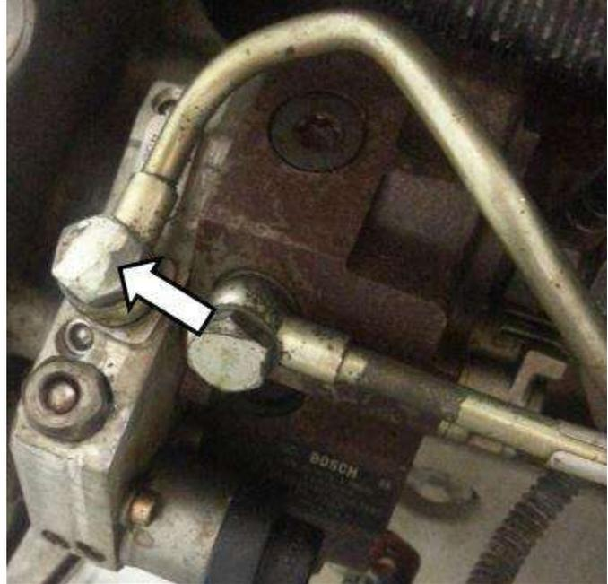
8. Pull the fuel bowl from the engine by removing the two bolts holding it in place using a 10mm Socket. Set these aside for re-install later.
