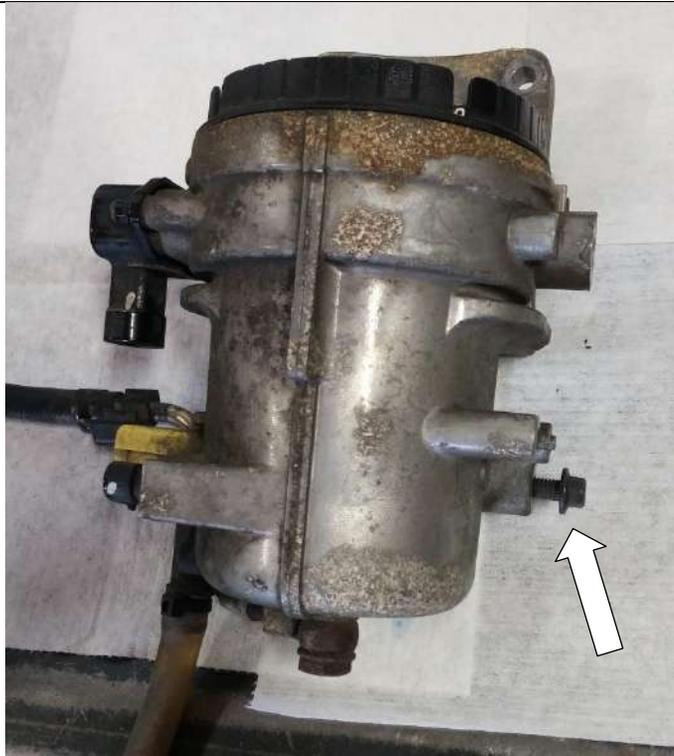
6. Loosen and remove banjo bolts from both sides of the fuel bowl with a 17mm socket. Set these aside, as they will be used later for install.
