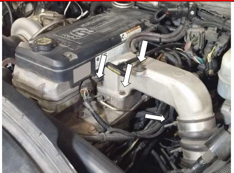
2. Place a pan or bucket below the fuel bowl and drain as much fuel out as possible by turning the drain valve. This will help reduce fuel spill when the fuel lines are disconnected.
