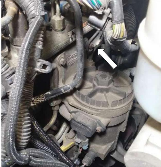
4. Disconnect the fuel heater and WIF sensor connectors.
