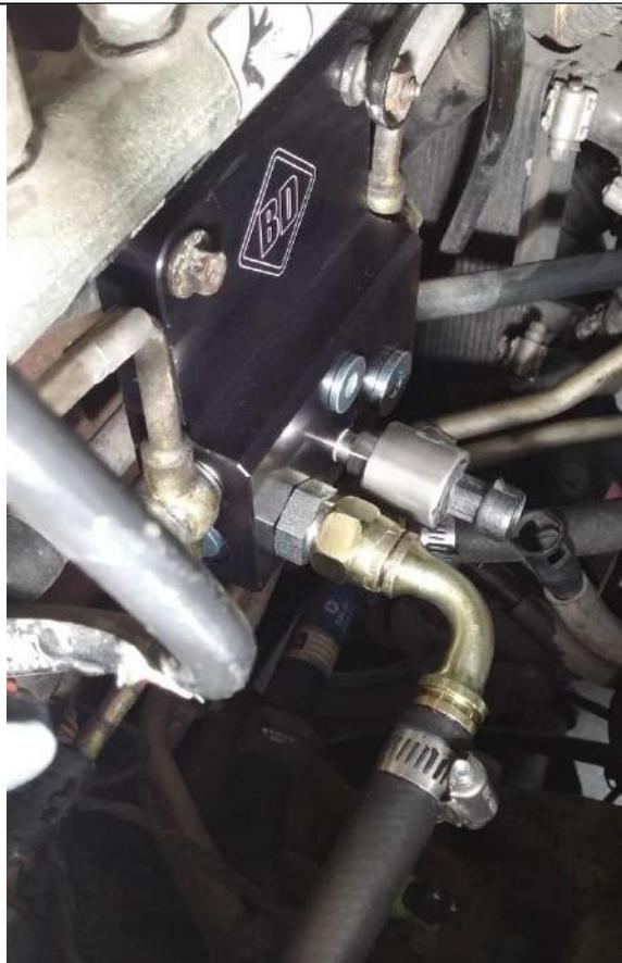
19. The connections for the factory WIF sensor and fuel heater will now be exposed. It is highly recommended that a WIF extension harness be installed into the factory connector to allow the use of an auxiliary WIF sensor.
