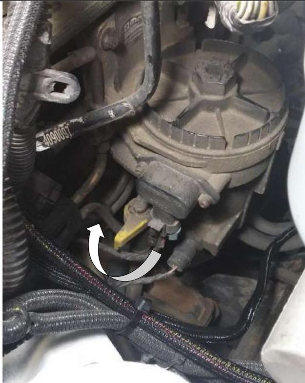
3. Remove dipstick mounting nut from the fuel bowl mounting bolt using a 10mm socket. (5.9L engine only)
