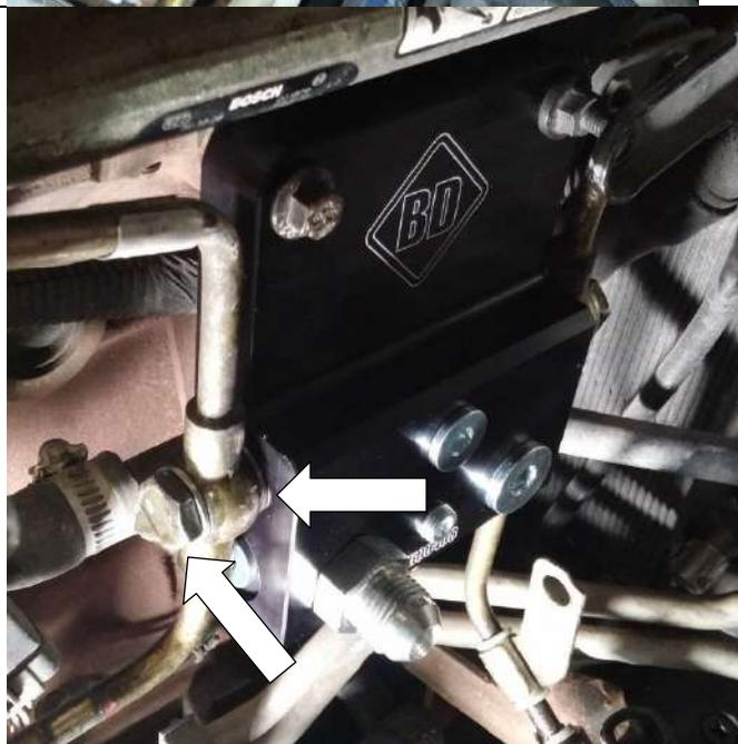
15. Tighten the two bolts holding the fuel distribution block to the cylinder head using a 10mm socket to **24 Ft-lbs.**
