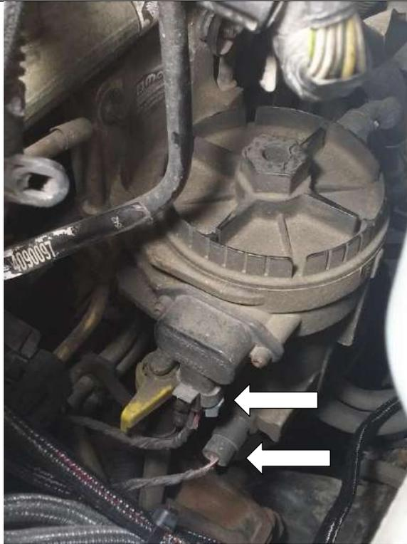
5. Remove bolt holding the return line to the back the of fuel bowl using a 10mm Socket. This fastener is not visible from the engine bay, and the bowl is shown removed for clarity.
