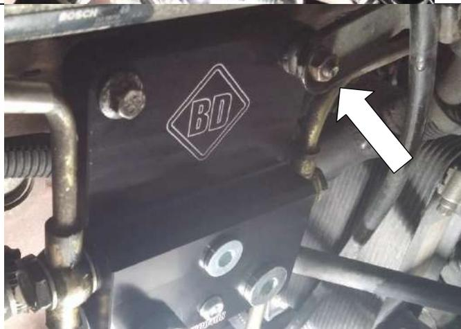
17. If running the fuel feed through the distribution block, attach the supplied swept -8 JIC to a 1/2" fuel hose (not supplied), and connect the hoses to their respective fittings.
