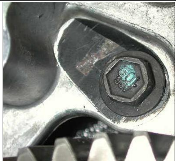
With retainer and bolt installed
