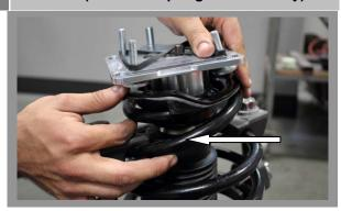
Place the Camber/Caster Assembly onto the Strut Assembly. <u>NOTE!!!</u> There is a supplied spacer for the 2005-2010 Mustang GT Models that needs to be placed onto the strut shaft before sliding the Camber/Caster Plate on.
