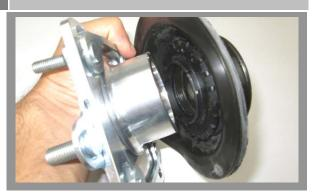
Install the Camber/Caster Assembly to the supplied Ford Strut Tower Pivot Assembly.
