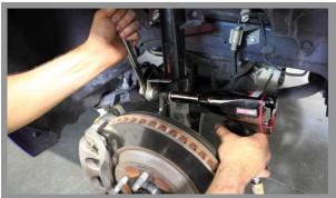
Remove the sway bar end link from the strut, then loosen but do not remove the strut mounting bolts.
