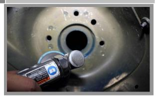
Check the bottom of the strut tower housing for any roughness. Use a Sander or sand paper to smooth out the Housing. <u>NOTE!!!</u> Must be smooth to allow the Camber/Caster Assembly to slide freely when adjusting.
