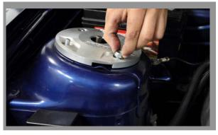
Re-install the strut assembly, place the cover over the strut tower where the studs protrude, don't fully tighten the top nuts. The factory strut tower brace can be used with this kit by placing the 2 ends above the decorative cover. <u>NOTE!!!</u>Remember to remove the rubber band holding the Camber/Caster Kit.
