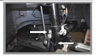
Remove the strut tower brace is applicable.
