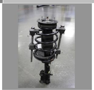
With a spring compressor, slowly depress the spring, then remove the upper strut retaining nut, then remove the upper strut mount assembly from the strut shaft. <u>NOTE!!!</u> Recommend the use of an impact gun.
