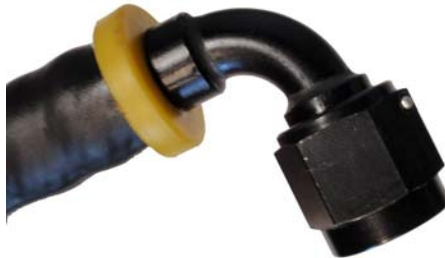
20 Hose ends pushed on
