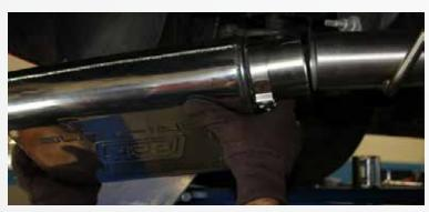
Slide the muffler with the adjuster towards the rear of the vehicle onto the inlet pipe and snug the clamp enough to still allow adjust-ability.
