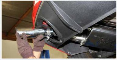
Slide the exhaust tip over the exit pipe and snug the clamp enough to still allow adjust-ability.
