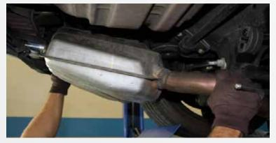
Slide the stock muffler towards the front of the vehicle and remove.
