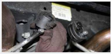
Remove the inner rubber grommets holding the muffler hangers.
