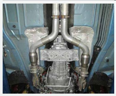
Now after headers are installed install supplied head pipe assembly the driver side and passenger side are labeled with little stickers on exhaust.
