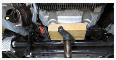
Safely support engine for removal and install motor mounts.
