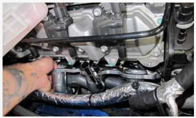
Install the BBK tune length header using the supplied gasket and hardware. NOTE the dipstick needs to be install at the same time by placing it through the header before putting it in.
