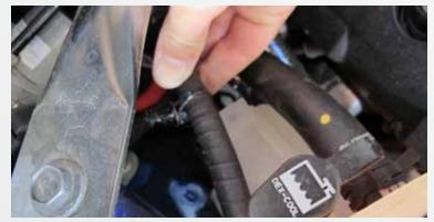
Disconnect the wiring harness from the reservoir bottle, remove the nut that secures the reservoir bottle to the chassis. Lift it up and it will lay up by the firewall.
