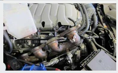
Remove the (5) bolts that secure the exhaust manifold to the cylinder head and remove it from the vehicle. NOTE the dip stick will come out with the exhaust manifold.
