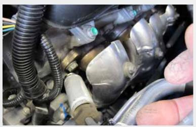
Remove the (4) spark plug wires from the coil packs and spark plugs.
