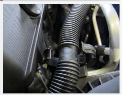
Disconnect the sound tube from the air box mounting point
