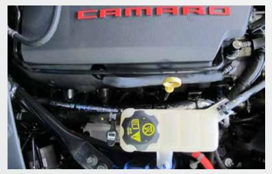
Connect the radiator hose to the reservoir, reinstall the wiring clip to the reservoir, install the valve cover, vacuum hose and engine cover.
