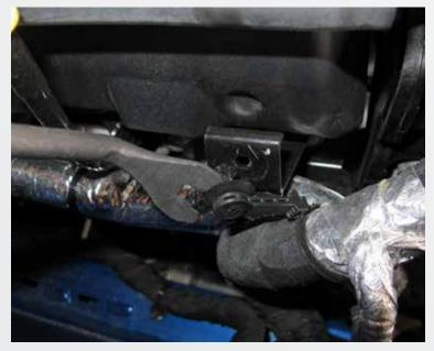
Disconnect the wiring harness from the engine bracket, remove the bolt that holds the wiring harness bracket in place and remove it from the vehicle.
