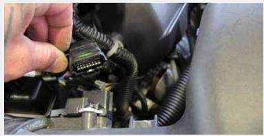
Unplug the wiring harness from the mass air sensor.
