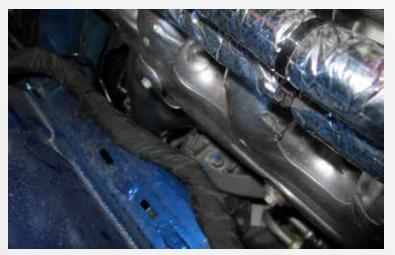
Remove the bolts that hold the upper portion of the heat shield to the stock exhaust manifold and remove it from the vehicle
