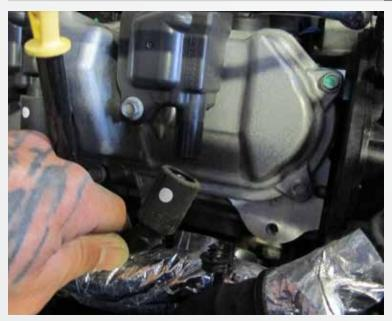
Remove the spark plug wires from the coil packs and the spark plugs.
