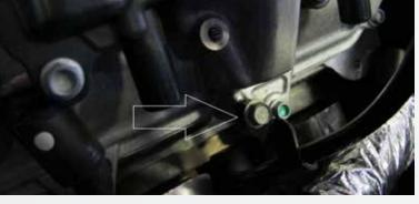
Remove the bolt that hold the oil dipstick in place.
