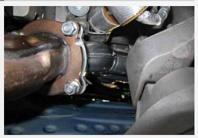
Install the supplied hardware to connect the catted mid pipe to the BBK tune length header and tighten it down, reinstall the steering shaft and tighten down its hardware.
