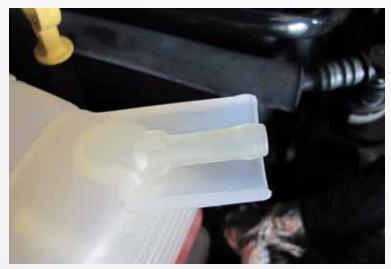
Driver side disconnect the upper radiator reservoir line from the reservoir using a bolt plug the end of the hose, using a rubber cap plug the reservoir bung.
