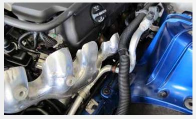
Passenger side remove the (3) bolts that hold the upper portion of the heat shield to the stock exhaust manifold and remove it from the vehicle.
