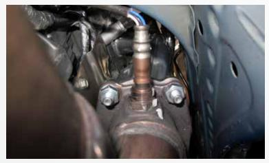
Install the (4) bolts supplied in the kit that connect the catted down pipe to the BBK tune length header and tighten them down.
