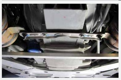
Tighten down the bolts on the cross brace. Reconnect the negative battery terminal after 500 miles of driving recheck and torque all hardware.
