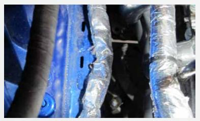
Tighten down all hardware on the header. Using the heat wrap supplied in the kit cover the lower wiring harness that runs along the body to protect it from any heat from the engine.
