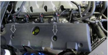
Remove the (2) torx bit bolts from the valve cover, disconnect the vent tube from the valve cover and the vacuum canister and remove the vacuum line and cover from the vehicle.
