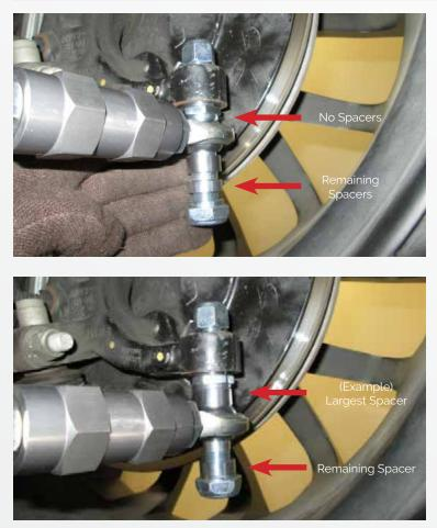
If the vehicle is at stock ride height then slide the tie rod end over the straight shank of the bottom of the tie rod stud then install the appropriate amount of spacers for tightening. If the vehicle is lowered you are going to want to install the appropriate amount of spacers between the spindle and rod end to achieve the measured angle from step 1, and then install the appropriate amount of spacers for tightening.
