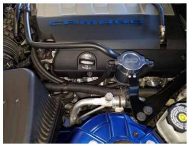
Remove factory strut tower bracket bolts then mount oil separator assembly, then run hoses forward and use supplied clamps at engine connection. Use 1/4 socket and ratchet to tighten clamps do not over tighten then use supplied zip tie for loose hoses as shown in picture.
