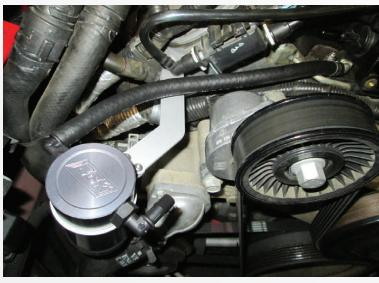
Start by running one hose from plastic fitting on intake manifold behind throttle body to the filtered side of oil separator this is the draw-side pulling crankcase pressure through filter and back to the intake. Then run the other side hose to the steel tube under intake manifold
