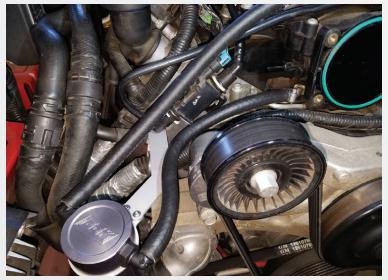
When running hoses to oil separator run your first hose from the plastic fitting on intake manifold to the filtered side of oil separator as shown in (pic). Then run the other hose from steel tube below intake manifold to the other side of the oil separator. This is the pressure side.
