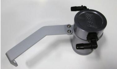
Assemble oil separator by installing o-ring bracket onto separator by removing cap. Now screw cap back down aiming towards top of BBK logo also install supplied fittings using 17mm wrench in the same direction. Now install bracket and alien bolts using a 3/32 alien wrench as show in photo.
