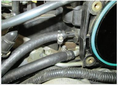
Now run the other supplied 3/8 hose to plastic port above steel one this is the return line from oil separator using clamp.
