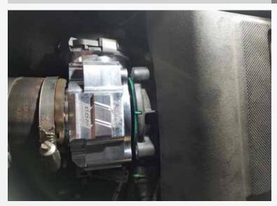
Install the BBK throttle body into the inlet hose and position it in place.
