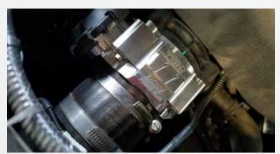
Reinstall the (4) bolts and tighten them down, install the wiring harness to the BBK throttle body and tighten down the hose clamp on the inlet tube to the throttle body, connect the negative battery terminal.
