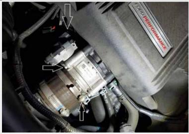
Disconnect the negative battery terminal. unplug the wiring harness from the throttle body, loosen the clamp on the inlet tube to the throttle body, remove the (4) bolts from the throttle body.
