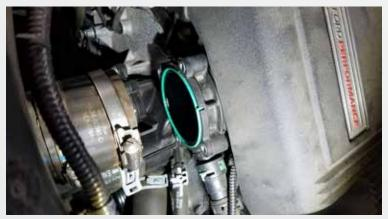
Remove the throttle body from the vehicle, wipe off any dirt or debris from the intake gasket before installing the BBK throttle body.
