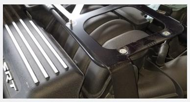
Disconnect the negative battery terminal, remove shaker from the vehicle if equipped to access the vacuum hose that will be replaced with the BBK oil separator kit.
