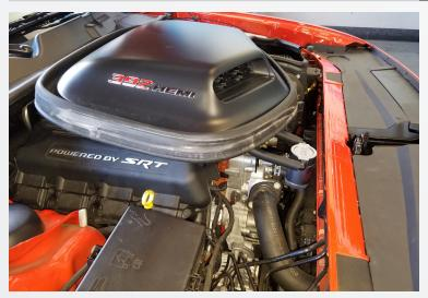
Tighten down all hardware and clamps, reinstall shaker if equipped, reconnect the negative battery terminal.
