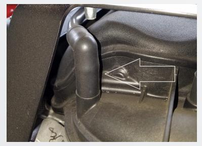
At the front of the engine disconnect the vacuum hose that is connected to the intake manifold.
