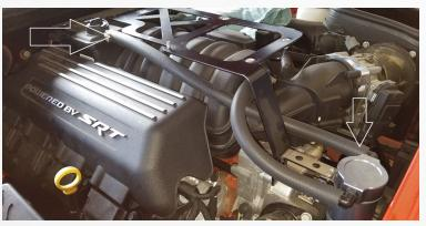
Using the longer vacuum line and clamp supplied in the kit install it onto the crankcase breather at the back of the engine, and connect it to the BBK catch can as shown in picture.
