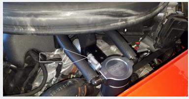
Remove the nut from the stud on the front of the engine install the BBk oil separator bracket onto the stud and reinstall the nut and tighten it down.
