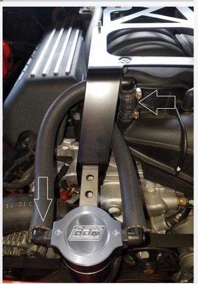
Install the BBK oil separator onto the bracket. Install the (2) shorter vacuum hose's and 90 degree fitting onto the intake manifold and to the BBK catch can as shown in picture.
