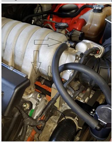
Install the vacuum hoses and clamps supplied in the kit. NOTE use the 90 degree fitting to connect the vacuum hose from the PVC to the BBK oil separator as shown in the picture.
