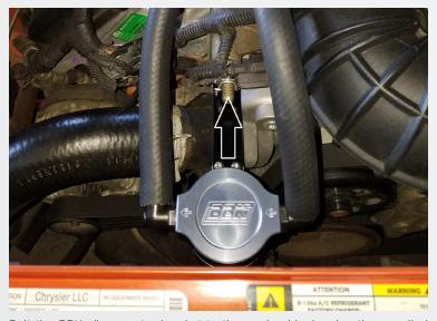
Bolt the BBK oil separator bracket to the engine block using the supplied bracket and hardware, install the BBK oil separator onto the bracket as shown in the picture.
