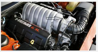
Disconnect the negative battery terminal. Remove the vacuum hose from the intake manifold that connects to the crankcase.
