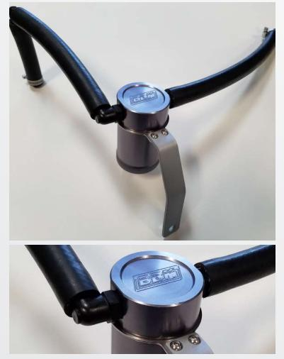
Now assemble complete oil separator kit as shown in picture. Making sure to use the two supplied hose clamps at valve cover and intake manifold connections only.
