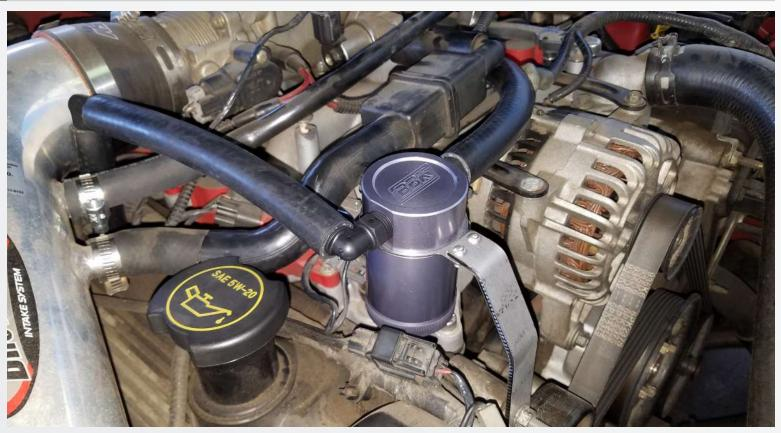
Now remove factory PCV hose that connects from the valve cover to intake manifold also remove 13mm nut next to idler pulley. Now install BBK oil separator kit mounting on factory stud and tighten as shown in picture. Use the two supplied hose clamps to clamp down hoses at valve cover and intake manifold.
