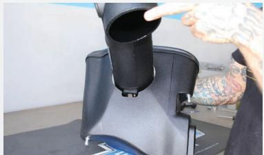
Now rotate the BBK tube anti-clockwise again until the mass air sensor location mounting area on the BBK inlet tube is positioned opposite the notch on the BBK airbox - now push/slide the inlet tube through again.
