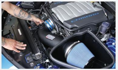
With the airbox installed and located - now we need to connect the rest of the inlet tube to the throttle body.
