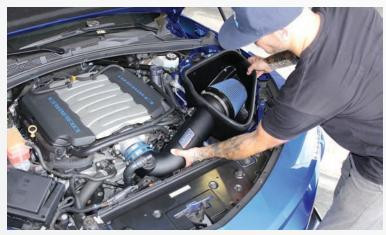
Now its time to install the complete BBK Cold air assembly onto the vehicle
