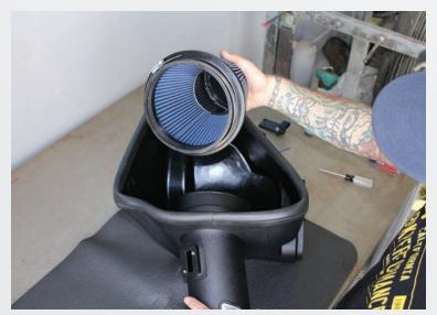
Time to install the air filter - Flat head screwdriver.
