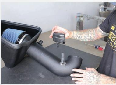
Install the black vacuum box onto the hose as shown.
