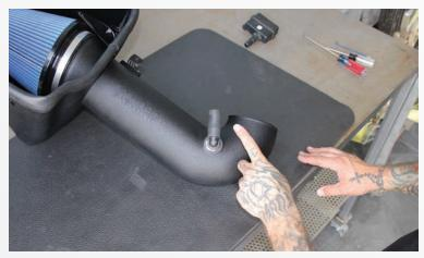
Screw in the fitting with hose attached all the way - once tightened move clockwise or anti clockwise until the hose is positioned as shown in the photo.
