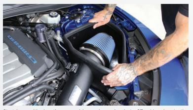
Start by positioning the assembly as shown in photo 27 – Now locate the metal locaters pins on the BBK airbox and locate the Black OEM grommets – when in position over each other – push down to engage and snap into position – locate the factory air inlet tube in the lower corner of the fender well and massage into position over the BBK airbox to allow the flow of cold air directly into the BBK airbox.
