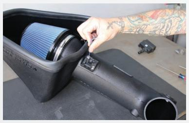
Use the 2 supplied screws to tighten the sensor to the BBK inlet tube in the mounting location.
