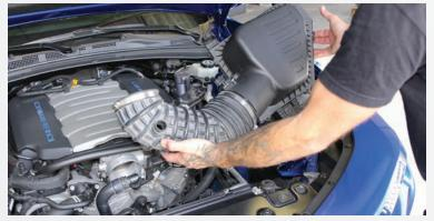
Once all free – it is time to remove the complete assembly as one unit as shown (remember to check that all the 3 Black rubber grommets on the actual airbox are in place in the cars locating positions. Check the box – if they have come off on the box when it was removed – pull them off and put back in position in the car where they were originally placed.
