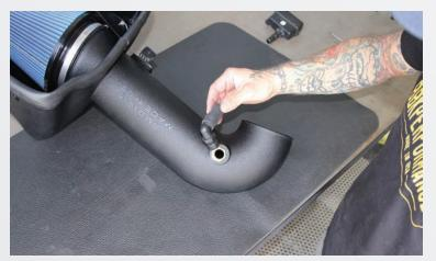
Now rotate the BBK inlet tube to show the underneath and you will now Install the supplied 90 degree fitting with the include supplied hose as show in the photo.
