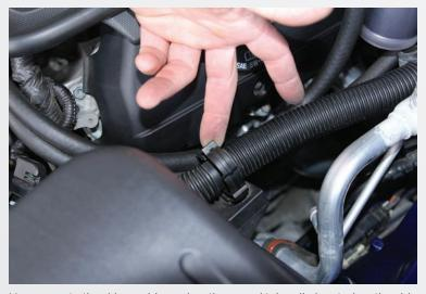
Now move to the drivers side again – the sound tube clip located on the side of the airbox assembly - Lift the tab on the clip and pull apart .
