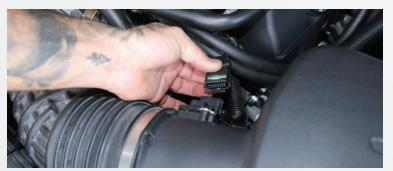
Disconnect the Mass Air Flow Sensor Harness by pulling back on the safety clip underneath – press and pull back – then move to one side.
