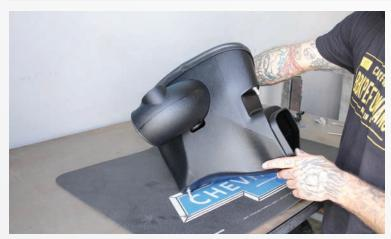
Now rotate the BBK tube anti-clockwise until the brass insert installed in the BBK inlet tube is positioned opposite the notch in the BBK airbox – now push/slide it until it is through.
