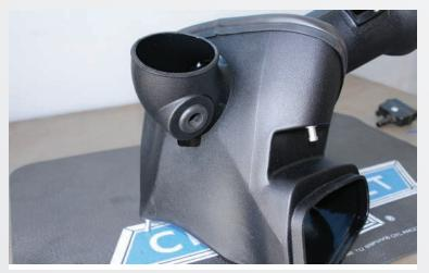
Take the BBK Inlet tube and position so that the front raised vacuum port area of the tube is opposite the cutout notch in the BBK airbox – now slide the tube through the notch (See photo).
