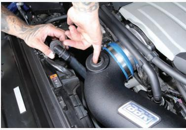
Apply a little light lubricant around and inside this grommet in the BBK inlet tube in front of the throttle body to ease the installation of the vacuum fitting. (See step 32).
