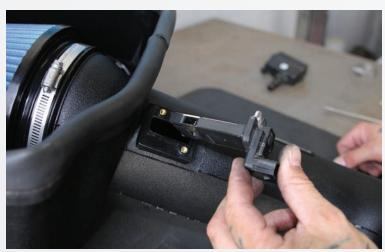
Install the OE Mass Air Sensor – attention: handle the sensor with care – no dirt or oil etc should be allowed to get near – this sensor is directional and will ONLY install one way – the opening/hole at the front of the sensor should be at the front (closest to the air filter as shown in photo).
