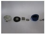
Once all the screws are removed loosen the C clamp slowly once there is a quarter inch gap between the two halves all tension is release proceed to unclamp and separate the two halves.
