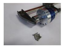
With the Fuel Regulator clamped firmly it releases then tension on the screws remove the six screws on the bottom of the Fuel Regulator.
