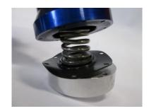
Place the spring cap on top of the spring with the pointed side facing down. With all the components together place the top portion of the Fuel Regulator on top. NOTE: While firmly holding the two half's together. Start the six screws into the bottom of the Fuel Regulator.
