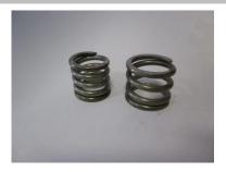
With the old spring taken out Its time to install the new spring supplied in the BBK Performance repair kit.
