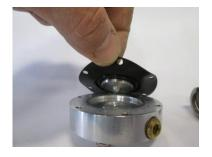
Place the diaphragm onto the bottom portion of the Regulator with the pointed end facing down.
