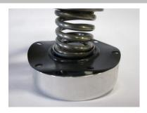
Take the new spring that is supplied in the kit and place it onto the spring locating cup on the diaphragm.
