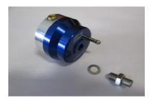
Remove adjustment screw and locking nut from the top of the Fuel Regulator .**NOTE:** Mark the two halves with a marker to indicate the orientation of the two halves. This way it will be clocked in the right position when put back together.
