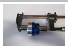
Using two 21mm sockets and a C clamp. Clamp the Fuel Regulator together firmly. NOTE: tape may be used on the two halves to prevent damage to the Fuel Regulator.
